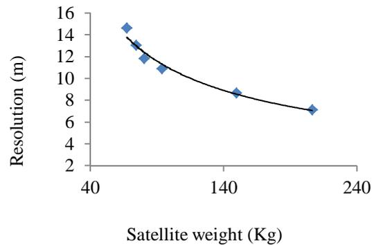
The variation of resolution with respect to the orbital altitude and weight of the satellite is shown in Fig. 5. The design space of the weight and resolution can be used as a decision making tool to help the designer make a balanced design decision among competing design objectives such as cost and performance.
