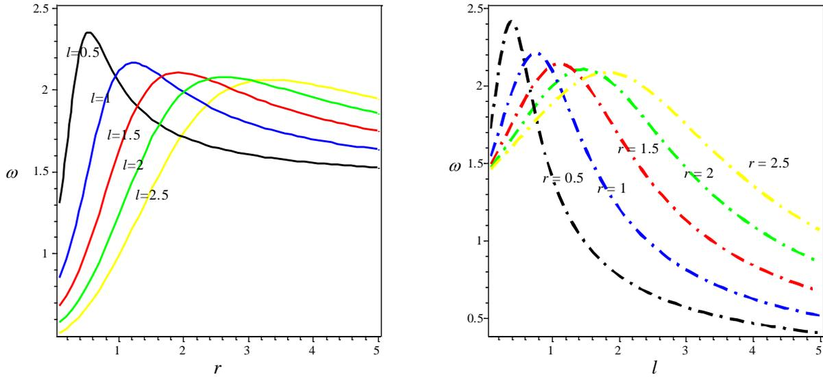
Fig. 3. Influence of axle length ( $l$ ) and radius of wheel ( $r$ ) on nonlinear frequency for  $m = 5, g = 9.81, k = 100, A = 10$
