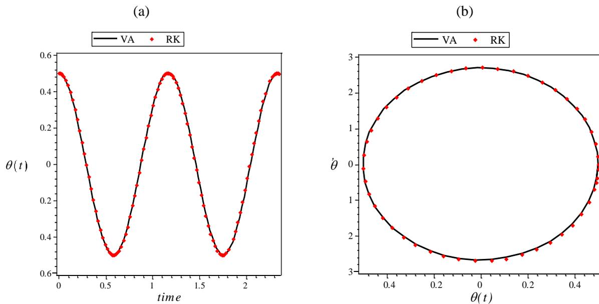
Fig. 2. Comparison of analytical solution of time history and phase curve with the numerical solution for  $m = 5, l = 1, r = 0.2, g = 9.81, k = 50, A = 2$
