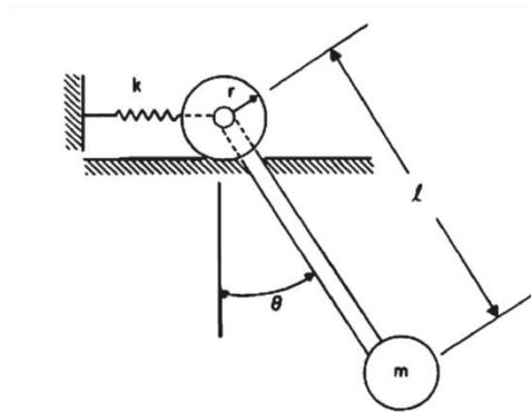
Fig. 1. Pendulum attached to rolling wheels that are restrained by a spring [23]
