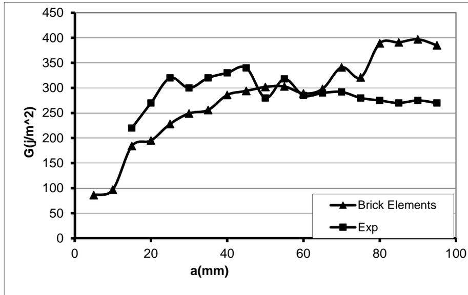
Fig. 13. Curves of strain energy release rate relative crack length for Brick elements
