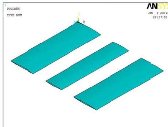
Fig. 2. Modeling of warps based on unit cell
