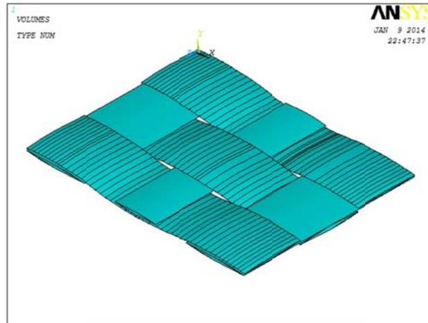
Fig. 6. Unit cell of fibres
