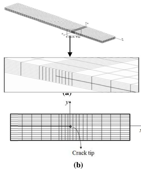
Fig. 8. Crack tip meshed with brick elements a) 3-D view [11] b) 2-D view in x-y plane
