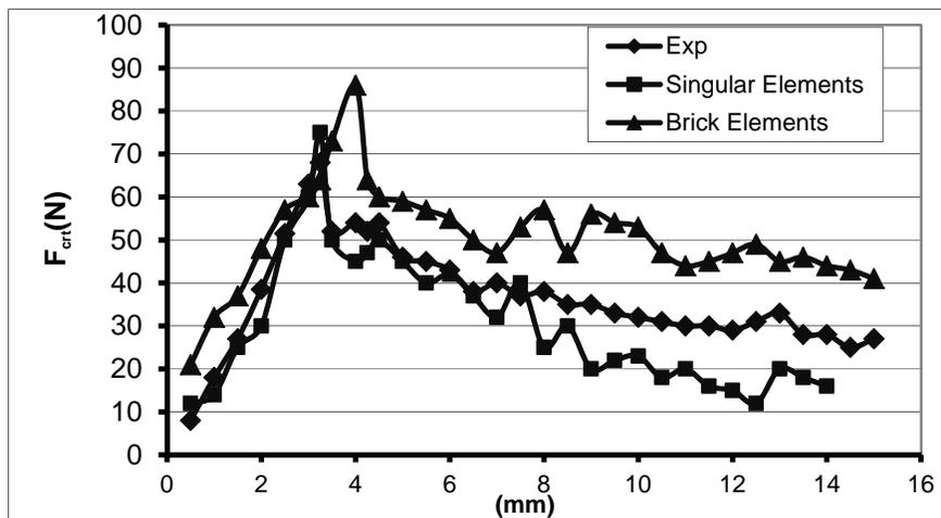
Fig. 10. Diagrams of load-displacement and comparison of numerical data with experimental data
