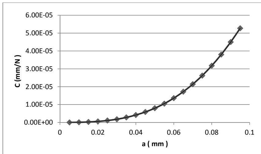
Fig. 12. Compliance versus crack length for singular elements
