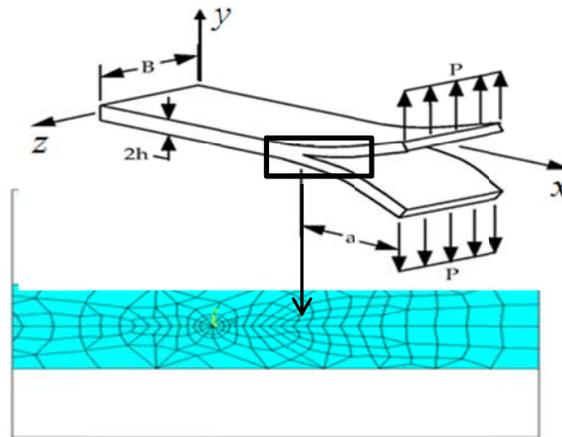
Fig. 9. Three dimensional mesh generation with singular elements on the crack tip [21]
