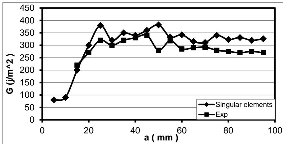
Fig. 14. Curves of strain energy release rate relative crack length for singular elements
