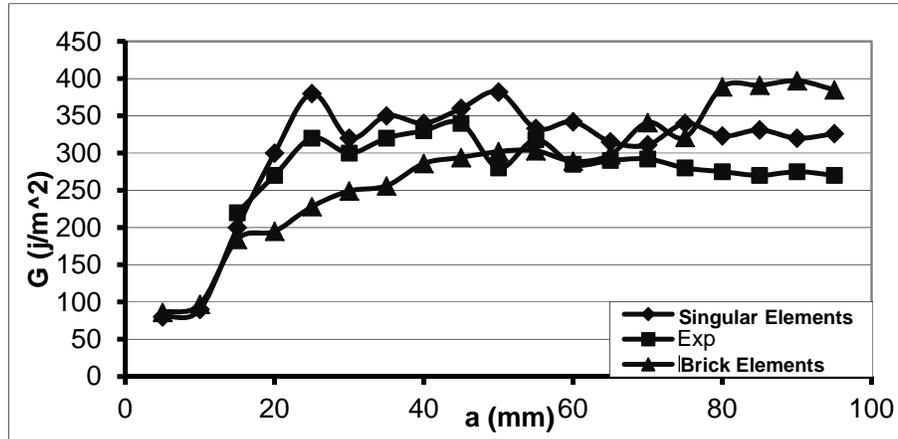
Fig. 15. Comparing the Curves of strain energy release rate relative crack length for types of elements
