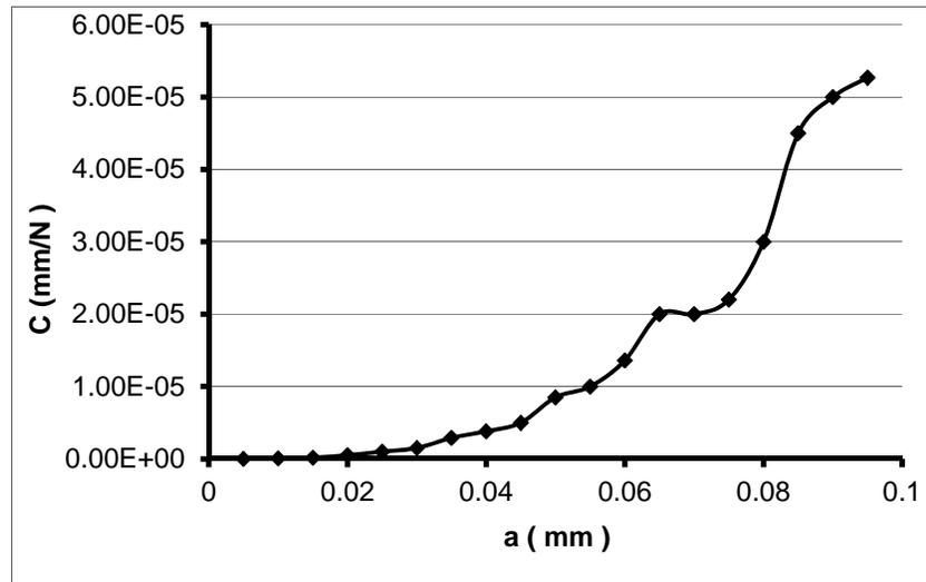
Fig. 11. Compliance versus crack length for brick elements
