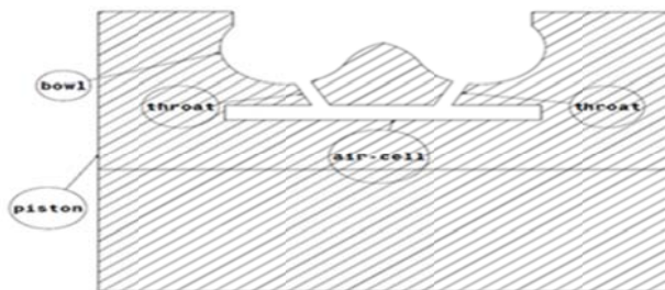
Fig. 2. Schematic view of modify piston
