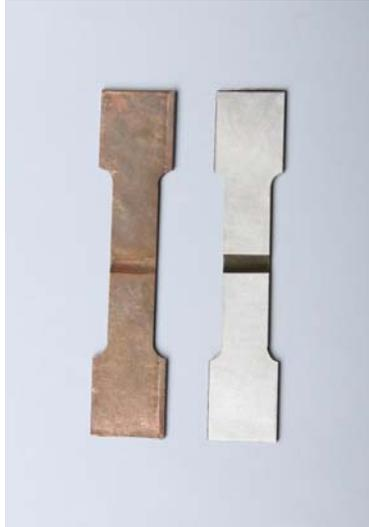
Fig. 4. The flat grooved specimen of copper/stainless steel clad sheet for determining the material damage parameters
